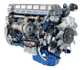
The D13K500 is a 500 hp, 12.8-litre, in-line, six-cylinder diesel engine equipped with an overhead camshaft, four valves per cylinder and common rail fuel injection. The engine meets the Euro 6 exhaust emissions requirements.
